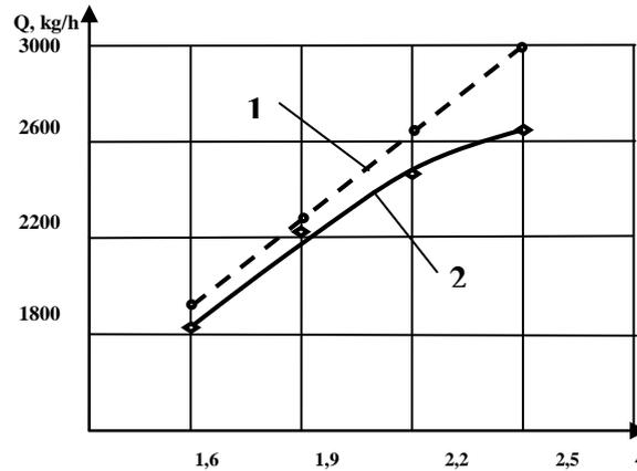
Figure 3: Dependence of capacity Q of the kinematic mode  $\lambda$ .
